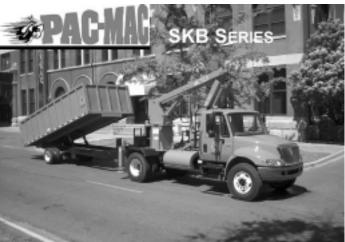
Pac-Mac is an original equipment manufacturer located in Bay Springs, MS. As part of the Hol-Mac Corporation our products include several models of knuckleboom loaders, trash trailers, dump bodies, and refuse bodies. With our primary focus on the knuckleboom line we offer options such as sit-down or stand-up operator, boom lengths up to 20' with bodies up to 25 yards. Our larger units have boom lengths up to 25' with bodies up to 40 yard capacity.
